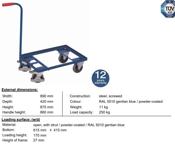
Wheelset: Ø 125 x 30 mm, thermoplastic rubber, grey, non-marking 2 swivel castors with brakes and 2 fixed castors deepgroove ball bearings More safety with the VARIOfit® foot protection
